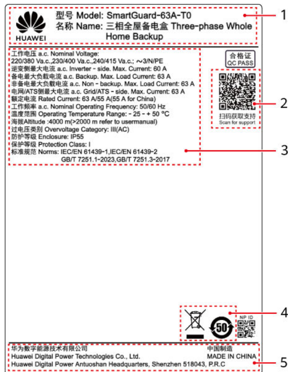
Figure 2-12 Nameplate (SmartGuard-63A-T0 as an example)
